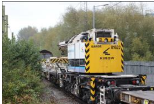
Figure 1: Kirow crane with a locomotive and trailers
