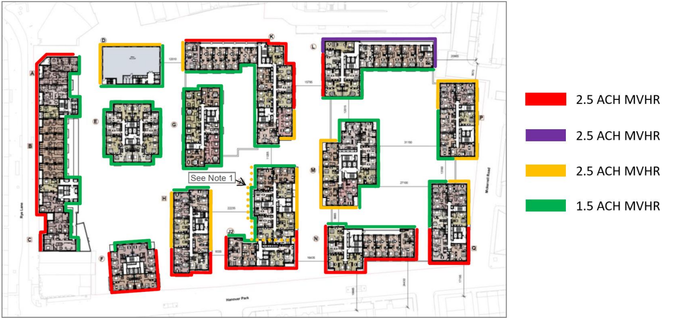
Figure 67 Apartments MVHR capacities
