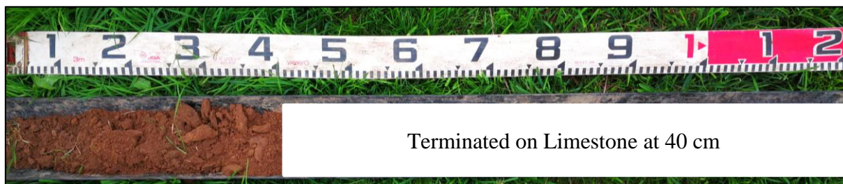
Photo 4. Borehole 3 – Soil Type 2*
