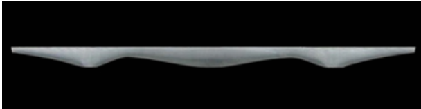
Figure 2.18: Concrete beam made with fabric formwork
