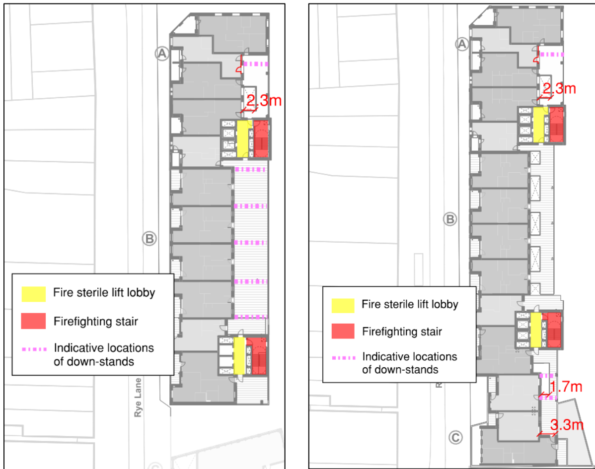
Figure 2 – External open deck of Building ABC at lower floors (Left: L1 and Right: L2)
