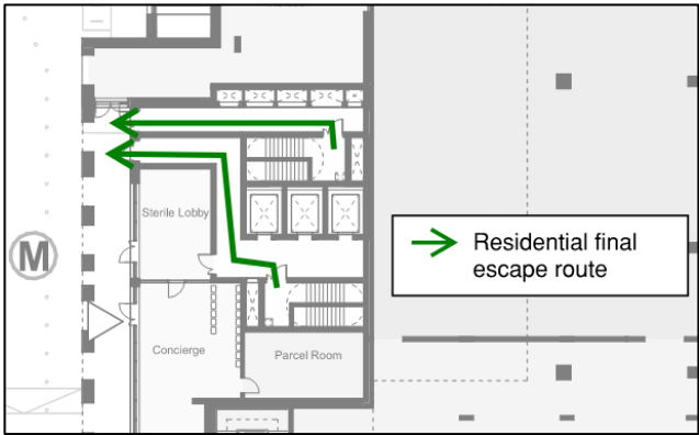
Figure 27 – Final escape routes of Building M
