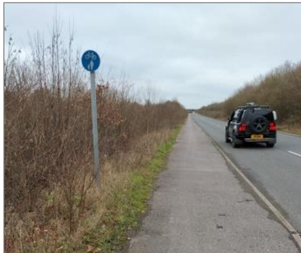
Image 2. Sign 956.1 must be used to allow horses to use the cycling/ walking path, not sign 956.
