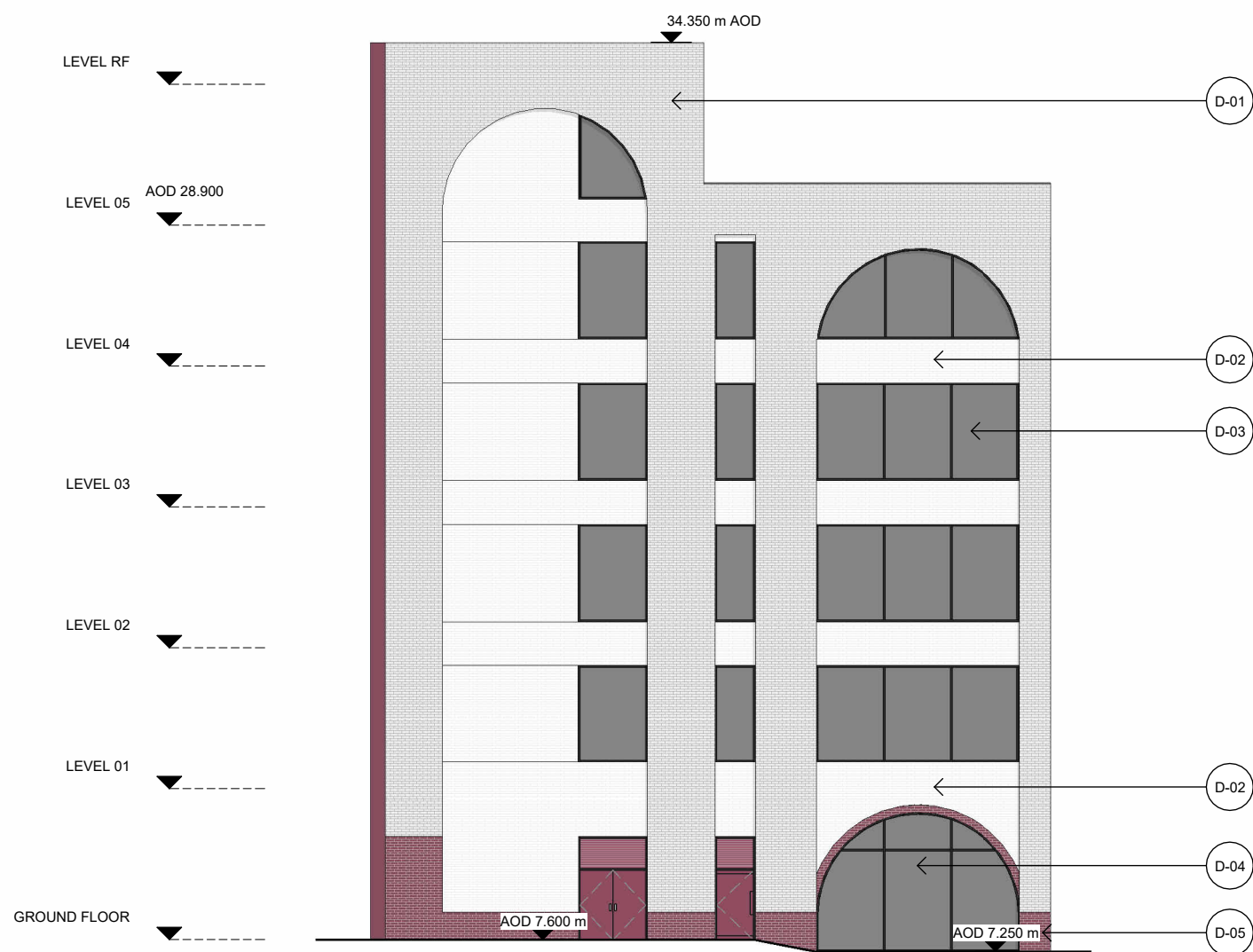
3 BUILDING D - EAST ELEVATION 1 : 200 Elevation
