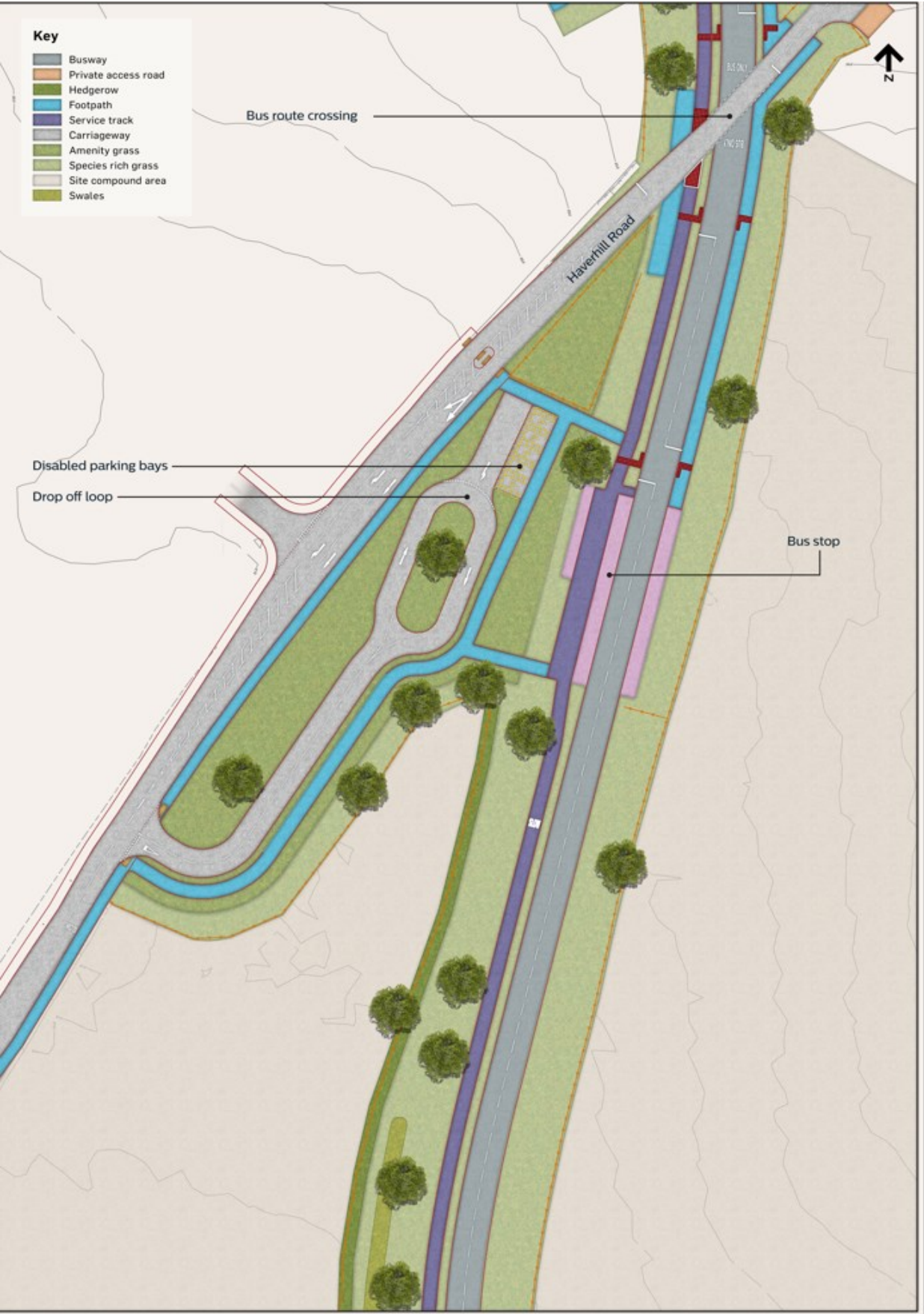
Figure 23: Busway route and crossing junction layout
