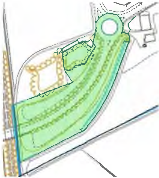
Figure 2 Extract of CCC Highway records confirming the ditch to the south of Addenbrookes Road is within the highway boundary.
