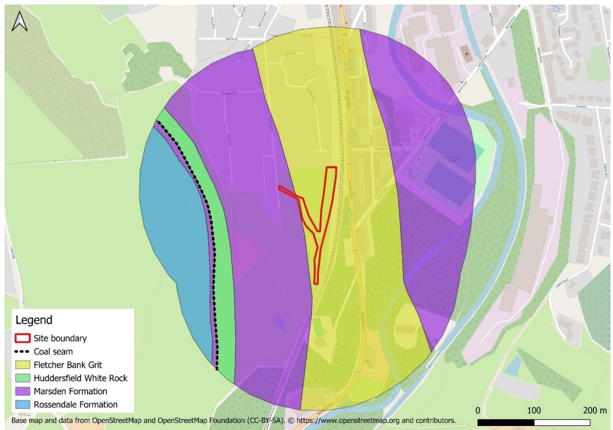
Figure 6-2 - Scout East Access work - Summary of bedrock and linear features
