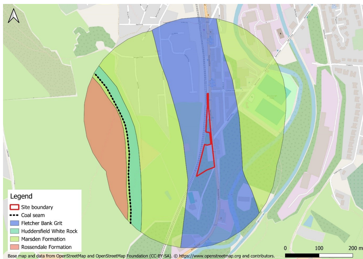
Figure 7-2 – Scout east laydown area and ramp access - Summary of bedrock and linear features
