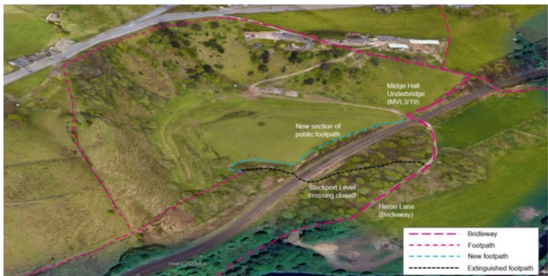
Figure 3-6 Proposed Stockport Road Level Crossing Diversion
