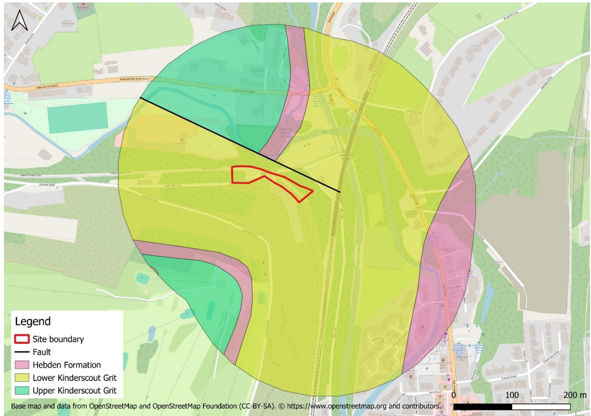
Figure 16-2 – Saddleworth viaduct vehicle access - Summary of bedrock and linear features
