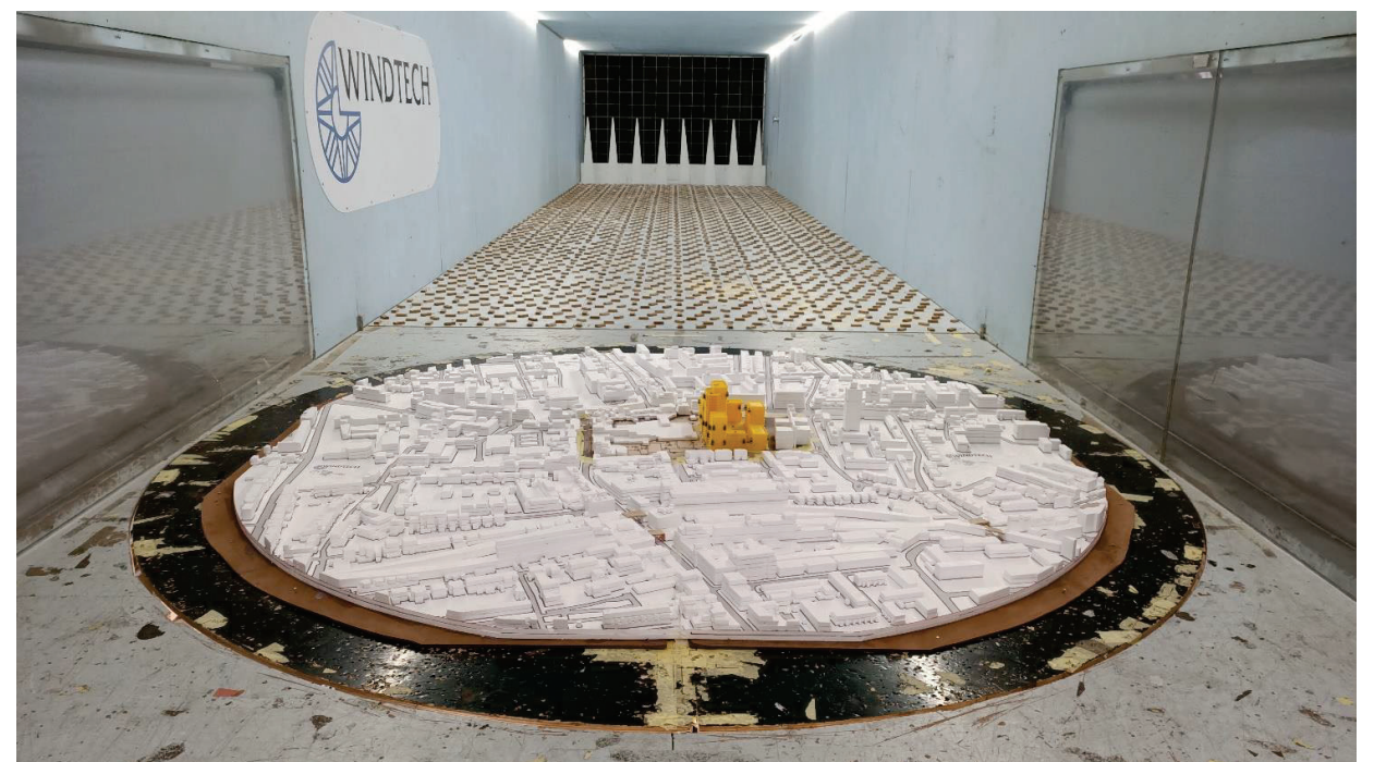
Figure 1b: Photograph of the Wind Tunnel Model: Interim Phase of the Proposed Development with Existing Surrounds (view from North)
