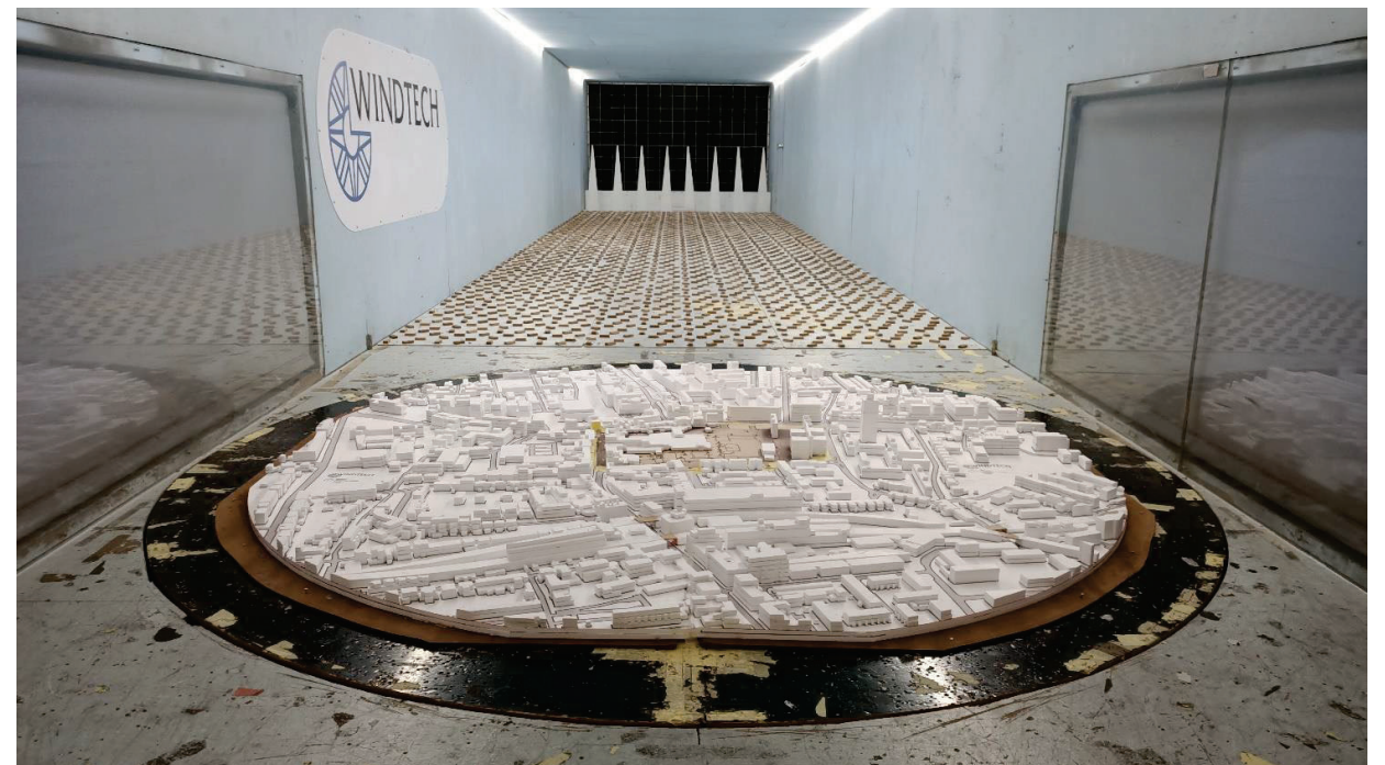
Figure 1a: Photograph of the Wind Tunnel Model: The Existing Site with Existing Surrounds (view from North)
