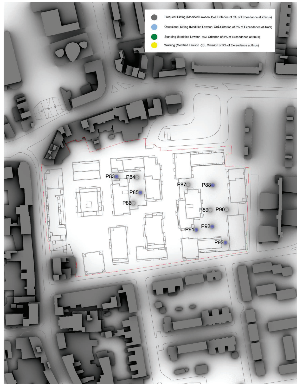
Figure 5b: Study Point Locations and Target Wind Speed - (Configuration 3) Completed Proposed Development with Existing Surrounds – Elevated Amenity
