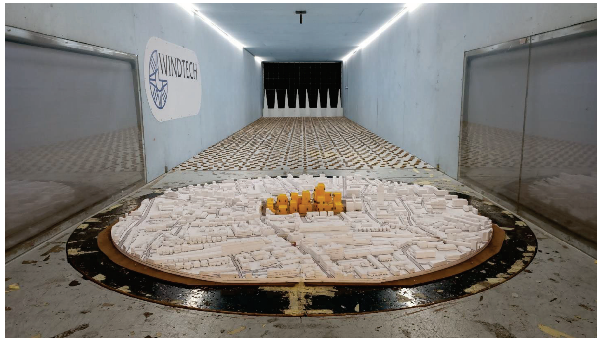
Figure 1c: Photograph of the Wind Tunnel Model: Completed Proposed Development with Existing Surrounds (view from North)
