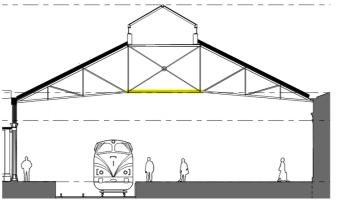
Figure 5.1.9.2b: Strengthening detail to bottom boom of 6No. trusses at Manchester end of Roof A
