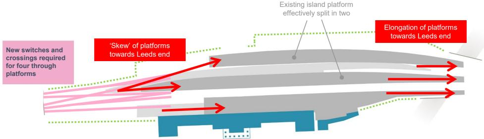
Figure 4.1.3a: Basic implications of track and platform alterations
