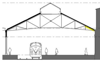
Figure 5.1.9.2c: Strengthening detail to top boom
