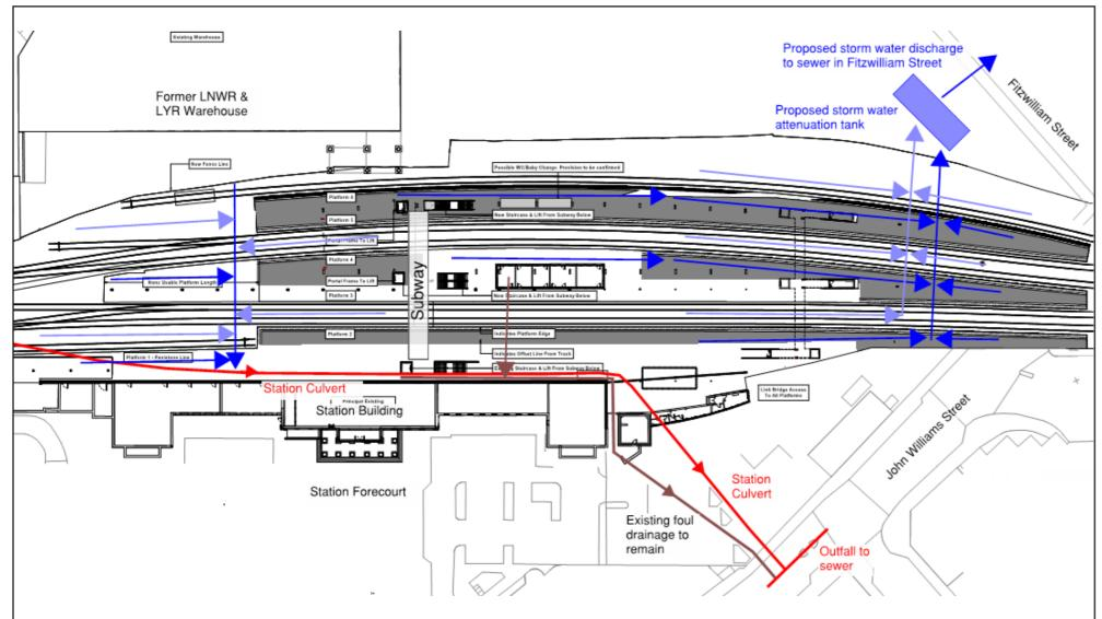
Figure 5.4.8.2a: Proposed drainage systems
