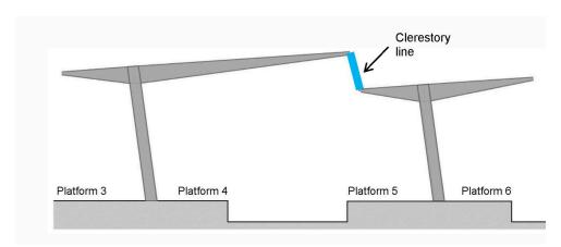
Figure 5.2.9b: Sectional view of the new roof at a column line
