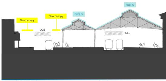
Figure 4.1.5d: Option 1 - new canopy coverage required (section)
