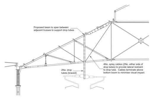
Figure 5.1.7a: Proposed OLE installation
