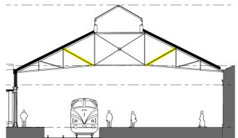
Figure 5.1.9.2a: Strengthening detail to diagonal elements
