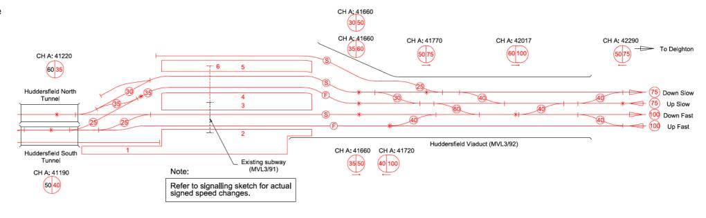
Figure 4.1.3b: Proposed schematic layout
