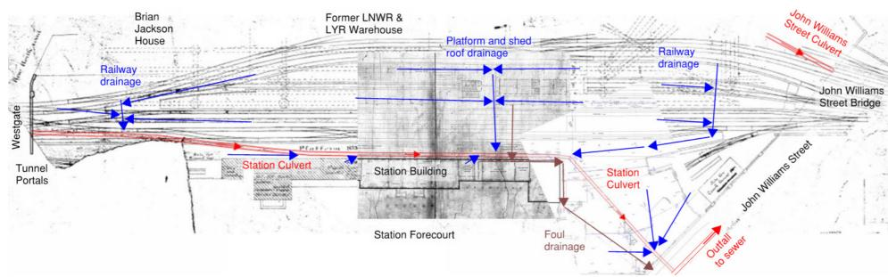
Figure 5.4.8.1a: Existing drainage systems
