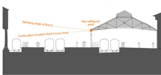
Figure 4.7b: Setting out lines derived from Roof A
