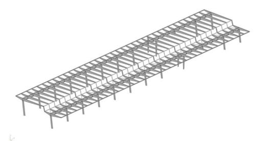
Figure 5.2.9a: Structural framing of the new roof (view from the North-West)
