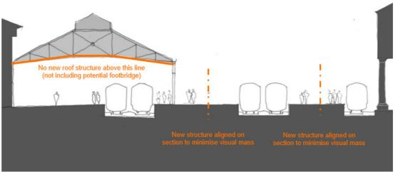
Figure 4.7c: New structure kept clear of Roof A gable; columns aligned on platform
