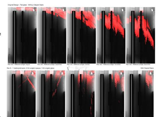
Figure 5.3.2b: Sun path study - flat glass (top) -v- sawtooth design (bottom)
