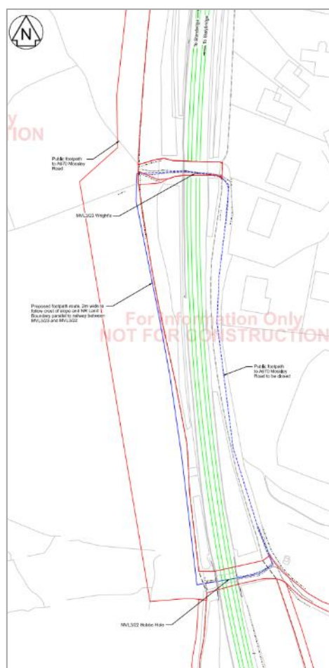
Figure 20: Wright's Overbridge (MVL3/23) PRow Diversion Plan
