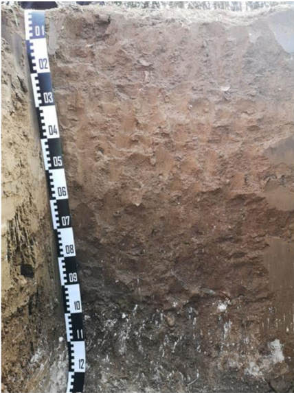
Figure 4.1.2: Inspection pit close to bore 26 within the Swaffham Prior Association. A well drained calcareous soil over chalk rubble. This example is atypically deep showing chalk drift at around 100 cms.
