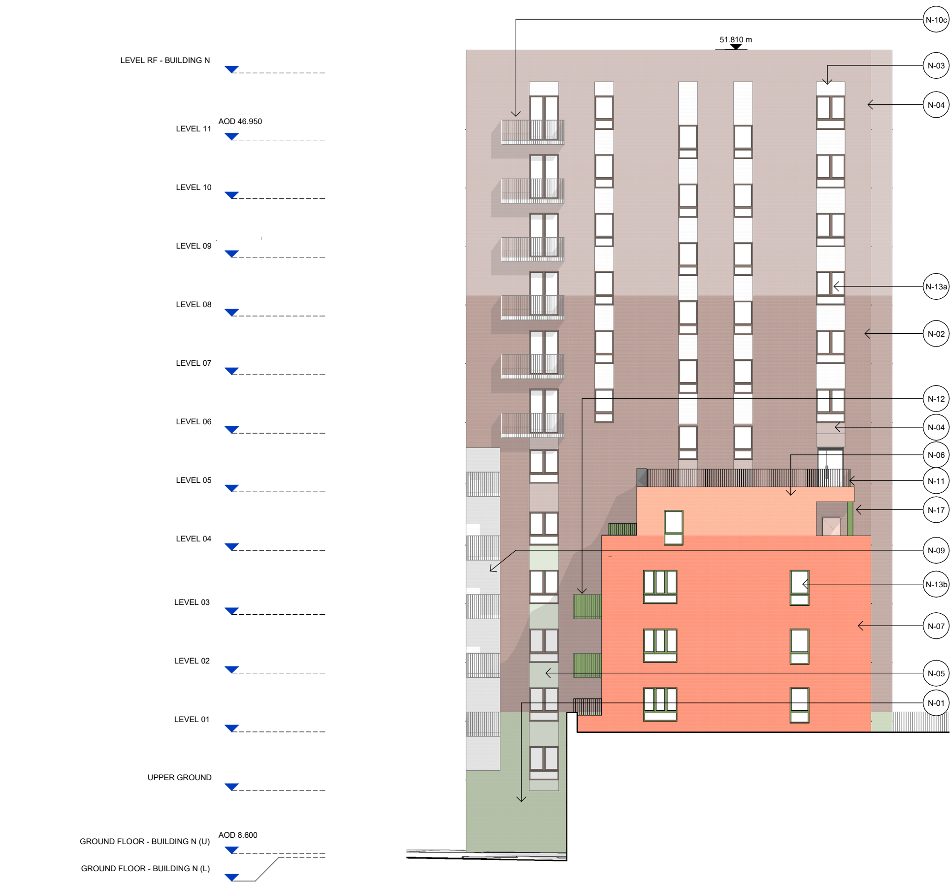
3 BUILDING N - EAST ELEVATION
