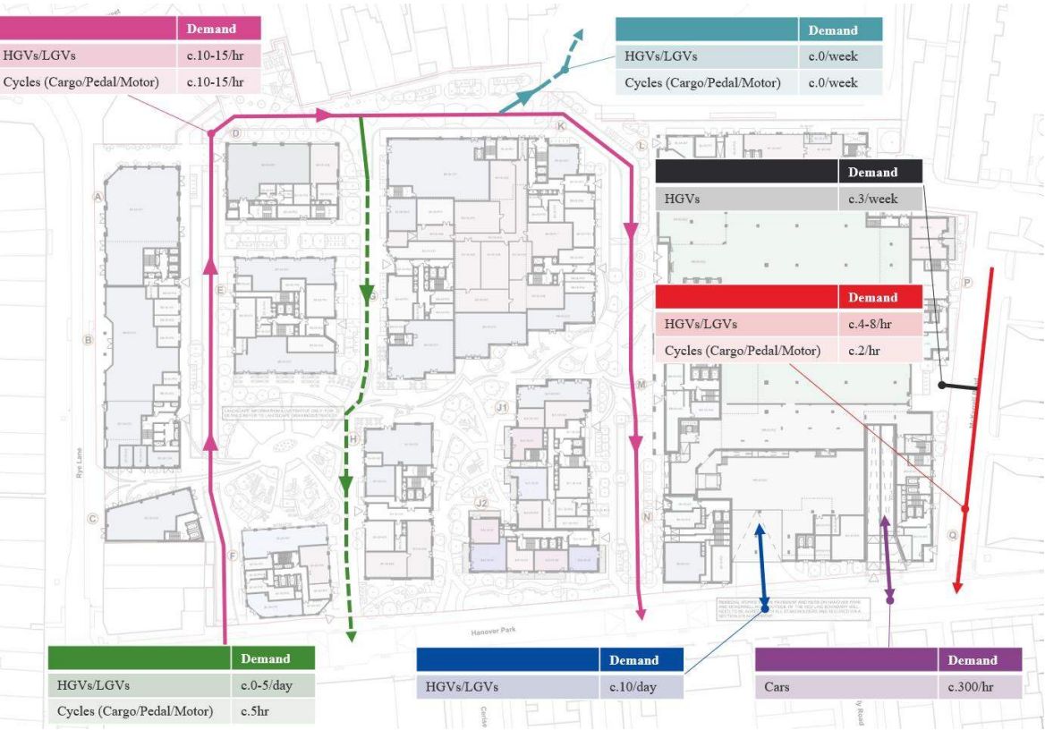
Figure 68: Typical Vehicle Movements (Two Way)
