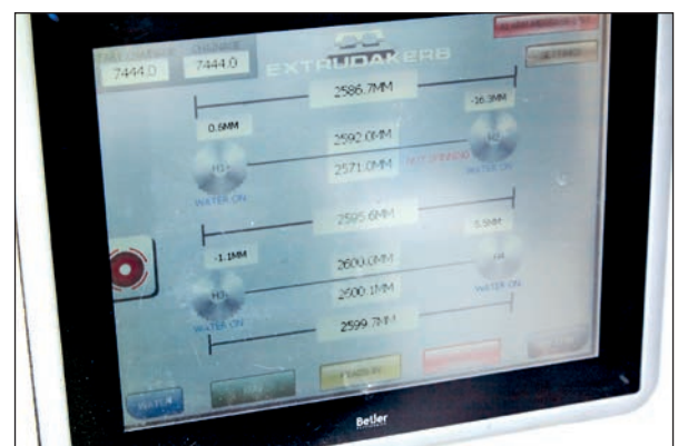
Figure 9.15 Gauge Readout from 2-stage grinding machine (Leigh & Ellenbrook busway) – Extrudakerb
