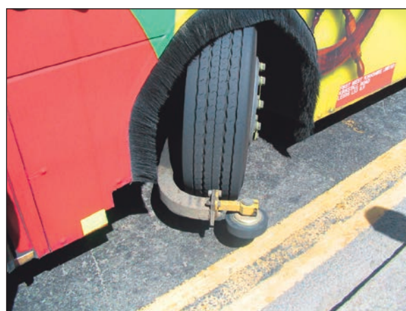
Figure 1.1 Guide wheel and arm on FirstGroup bus, Leeds (Scania 3-series chassis)
