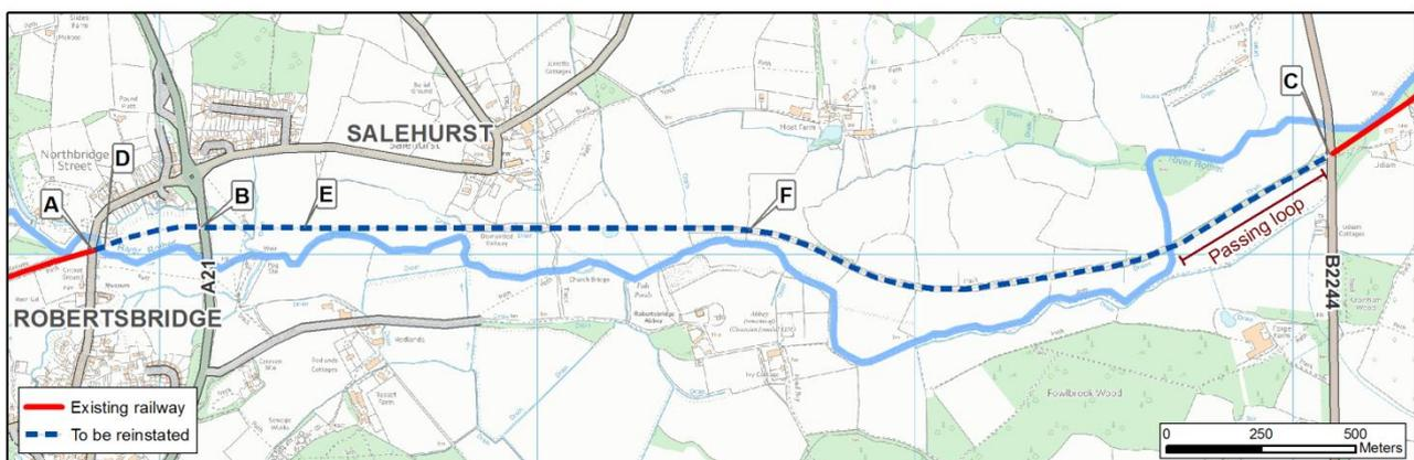
A new halt (Figure 1- Point F), which is a minor stopping place, is proposed to be built alongside the railway which would serve the village of Salehurst. There will also be a short section of double track railway that would serve as a passing point for trains travelling in opposite directions, this would be located adjacent west of the B2244 (as shown in Figure 1).
