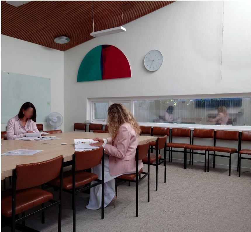
Figure 10 Existing meeting room illustrating the deliberate lower placement of the window cill so that views can be seen while seated at the meeting room and study desks
