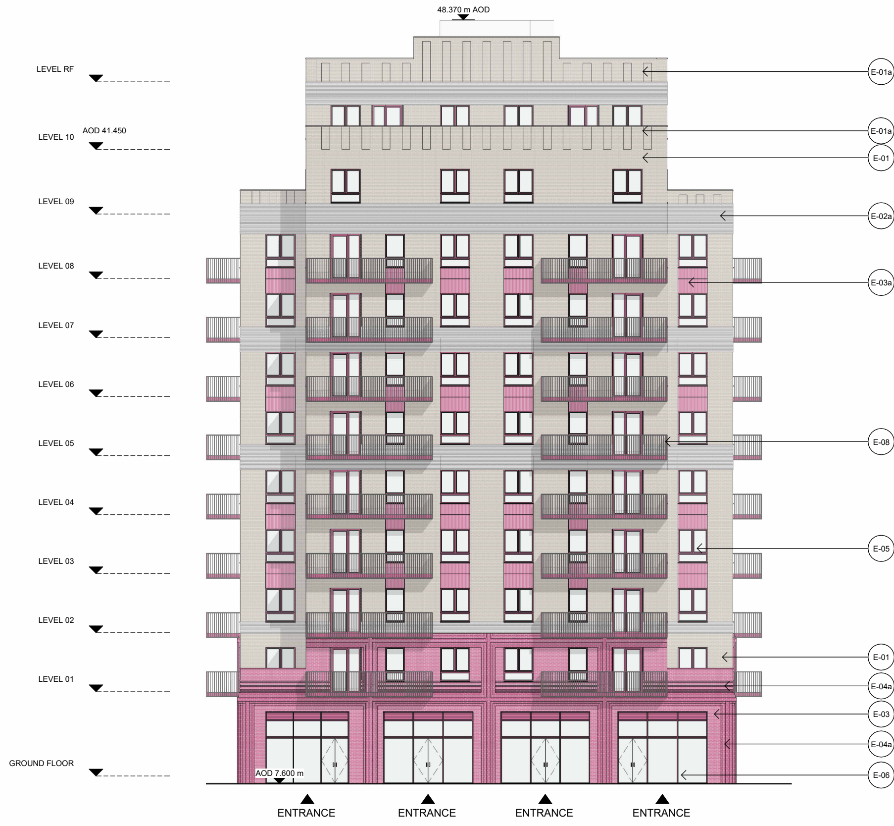
2 BUILDING E - NORTH ELEVATION
