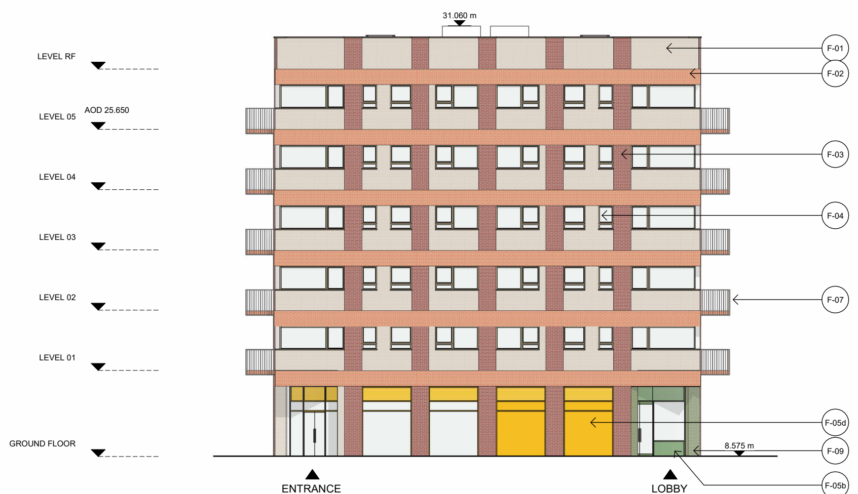
4 BUILDING F - F_SOUTH ELEVATION
