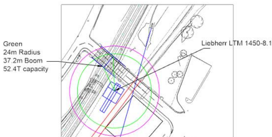
Figure 19: 500T crane position at track level
