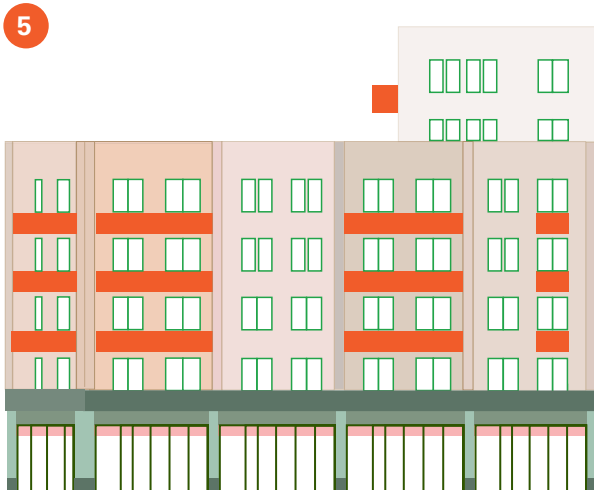
Openings following historic precedent
