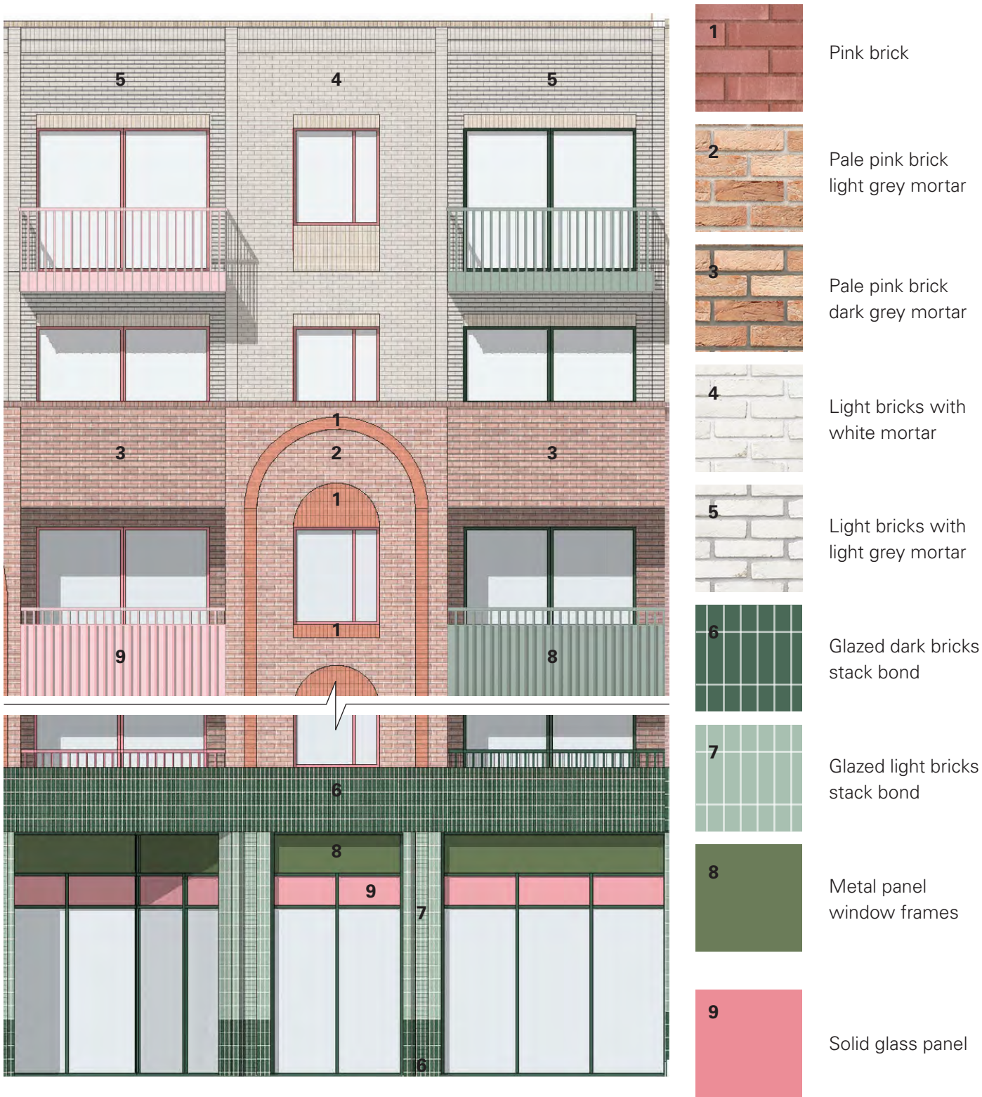
Building B - Bay study, west elevation
