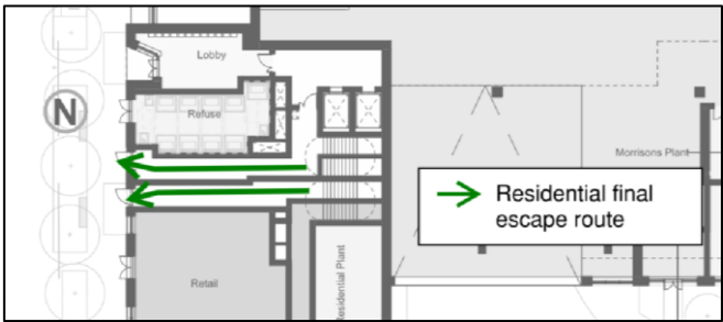
Figure 28 – Final escape routes of Building N
