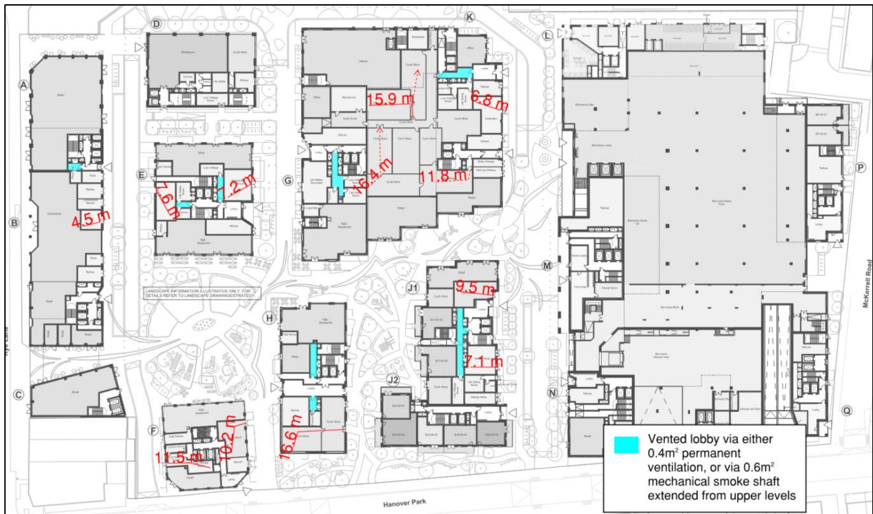
Figure 42 – Travel distances of ancillary accommodation at ground
