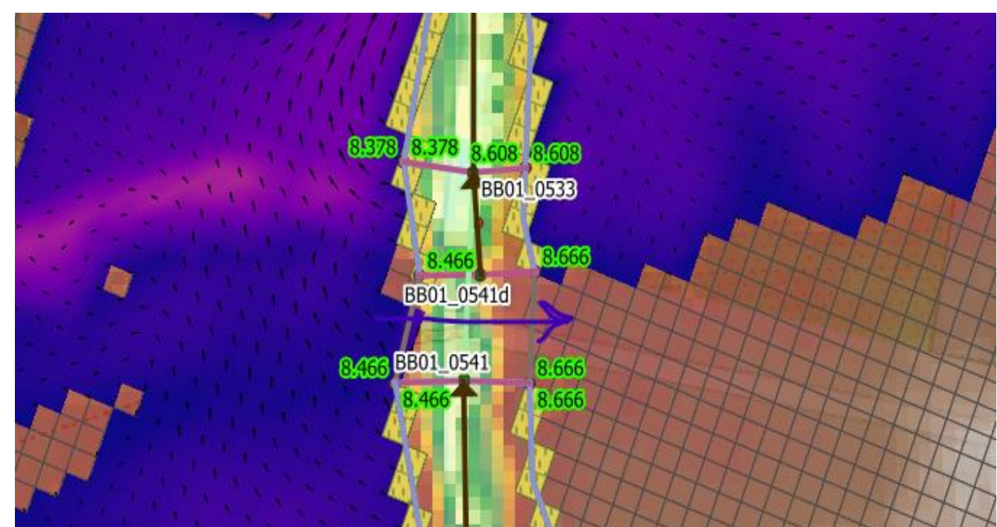
Figure 10: Weir looks to be sharp crested model with default broad crested coefficient
