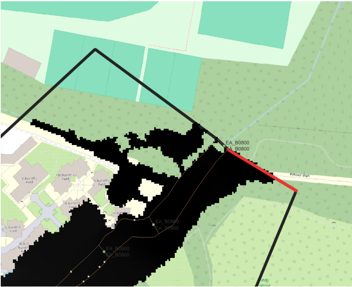
Figure 3: glass walling at the downstream left bank where no HQ boundary has been applied.
