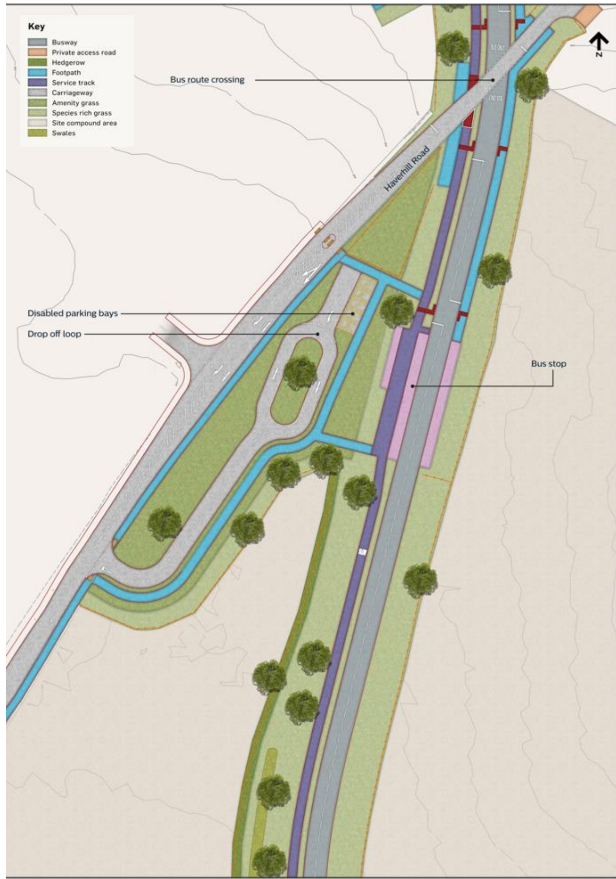
Figure 23: Busway route and crossing junction layout
