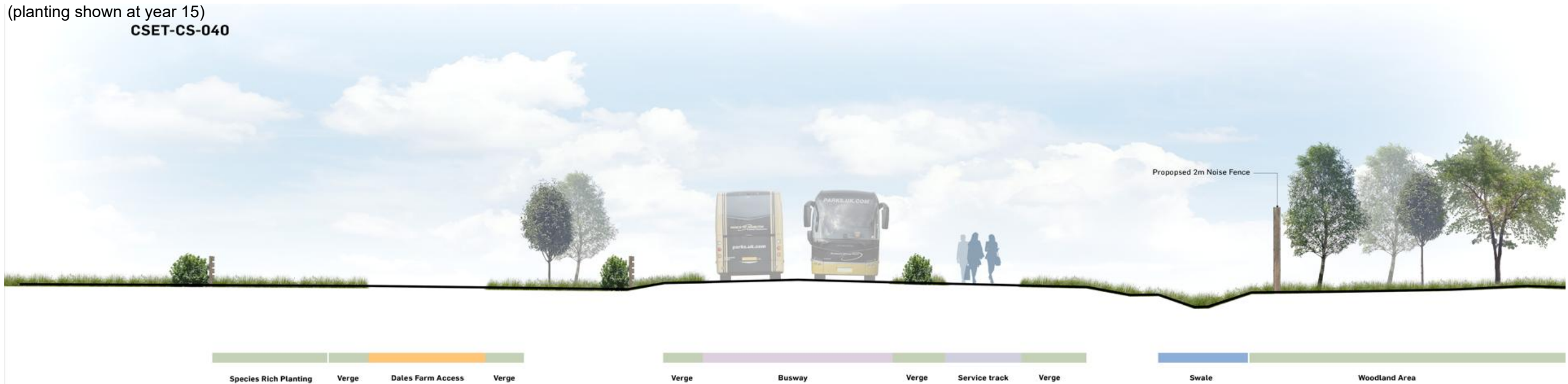
Figure 40: Typical section showing the proposed busway, proposed woodland, noise barrier and the Hawthorns (new residential development)
